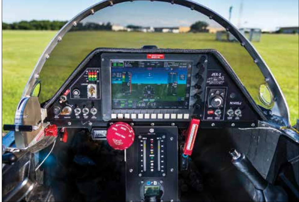
The SubSonex panel is dominated by a single EFIS screen. Very few switches are required for the rest of the plane's operation. The engine monitoring panel is in the center console.
