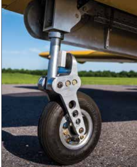
(Left) The landing gear indicators are LEDs located above the simple toggle switch. (Center) The steerable nosegear is custom built by Sonex and fits the jet perfectly. (Right) The main gear features two tires per side—just like the space shuttle. To improve stopping power, John Monnett has a new design in the works for the brake system.
