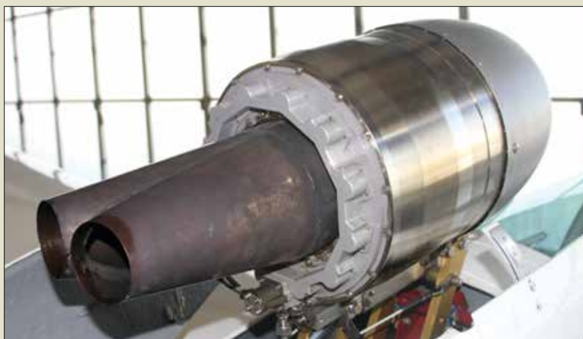
The key to the BonusJet is the PBS TJ-100 engine—in this installation using a bifurcated nozzle to avoid the vertical fin on the Bonus airframe.
