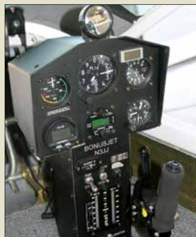
The instrument panel on the BonusJet is standard glider—except for the jet engine monitoring panel at the bottom.
