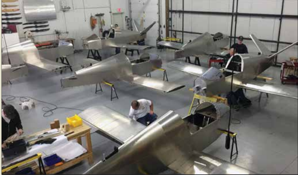
SubSonex quickbuild kits under construction in Sonex's Oshkosh facility. Despite the caché of being a jet, the construction is familiar to anyone who has built a Sonex.
