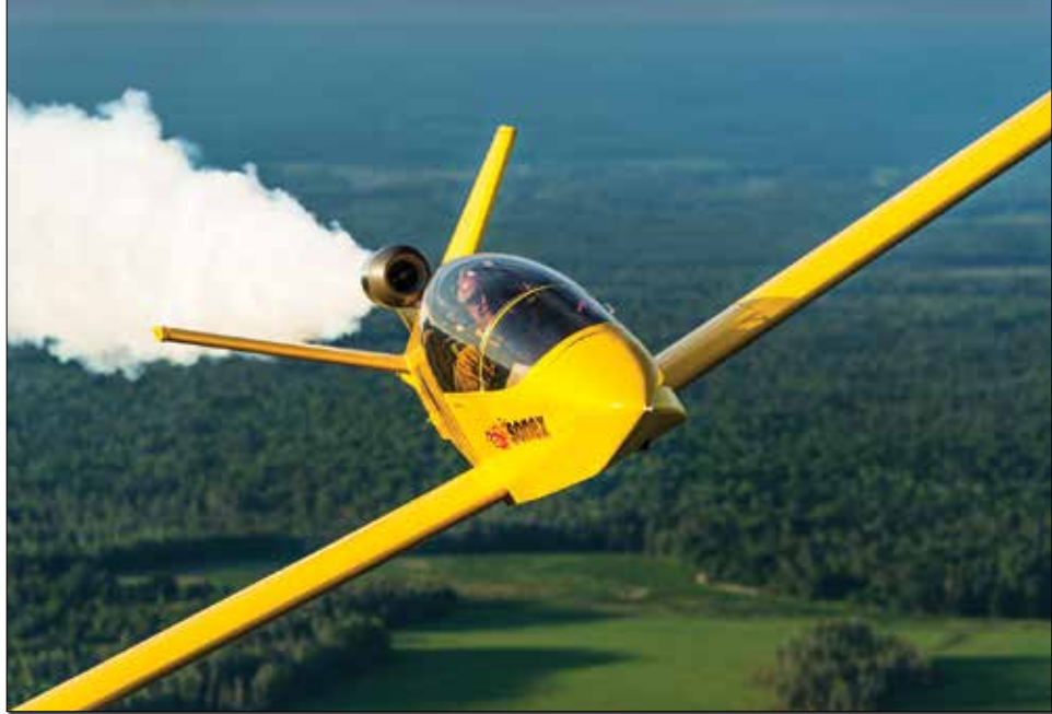
With no room for a standard smoke tank, Carlton designed a conformal fiberglass container that fits in place of the seat cushions for airshow work. It is quickly removable for normal flying.
