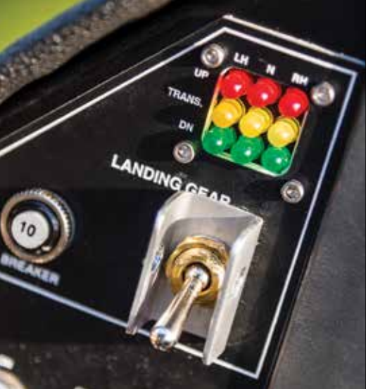
(Left) The landing gear indicators are LEDs located above the simple toggle switch. (Center) The steerable nosegear is custom built by Sonex and fits the jet perfectly. (Right) The main gear features two tires per side—just like the space shuttle. To improve stopping power, John Monnett has a new design in the works for the brake system.
