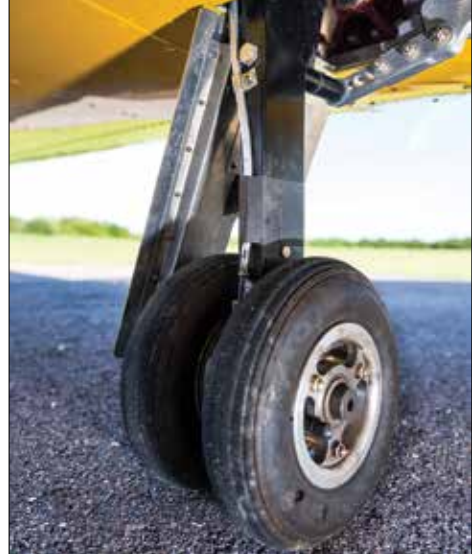
(Left) The landing gear indicators are LEDs located above the simple toggle switch. (Center) The steerable nosegear is custom built by Sonex and fits the jet perfectly. (Right) The main gear features two tires per side—just like the space shuttle. To improve stopping power, John Monnett has a new design in the works for the brake system.
